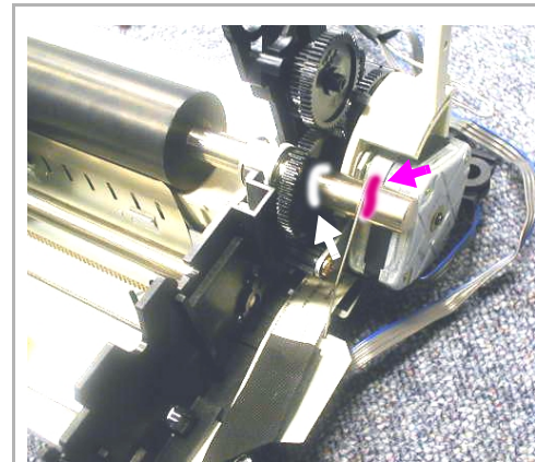
Figure 6-12. Platen Grounding Spring / Spur Gear
